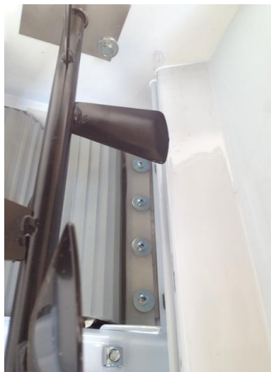
Fig. 3 Detail of the inside of the hopper and the rollers
