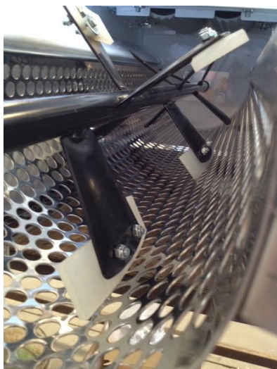
Fig. 2 Detail of the basket and flap mixer
